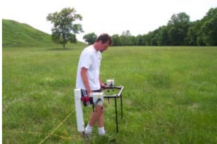
Figure 9. Jon Kerr surveying portions of the Workshop Grid with duplex Geoscan Research fluxgate gradiometers.
