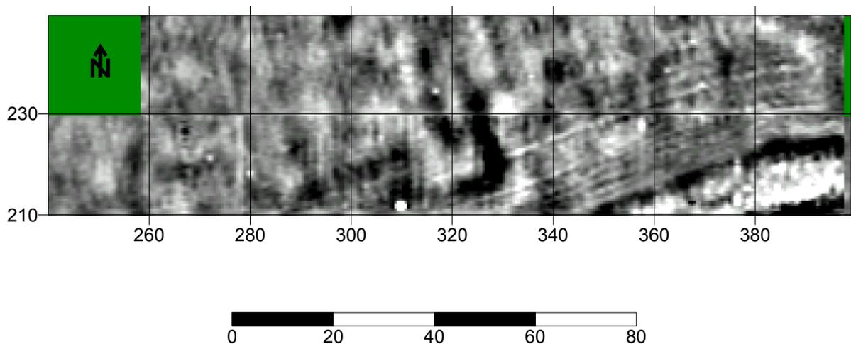
Figure 8. Effect of Multiple Low Pass Filterings on the Conductivity Data.
