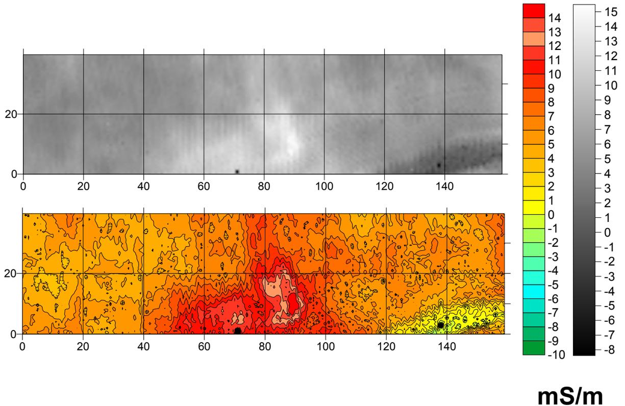
Figure 3. Surfer 7 Gray Scale and Contoured Images of Workshop Conductivity Data.
