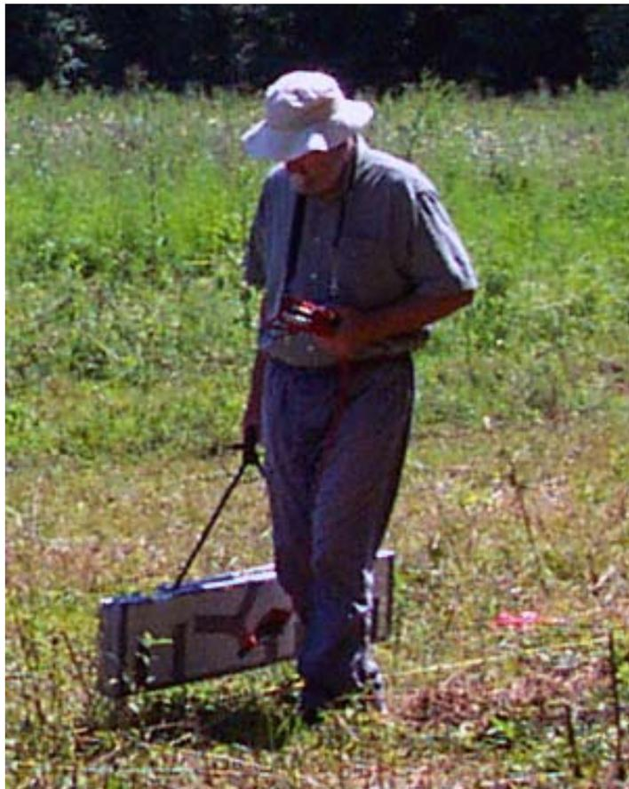
**A Conductivity Survey in Progress.** The EM38 is carried in the right hand, ca 15 cm off the ground. It is contained in a sheath of foam insulation held together with Duct Tape (!). The data logger is carried in the left hand and manipulated with the left thumb. Not so obvious is the marked rope below the EM38, the object of the author's rapt attention.
